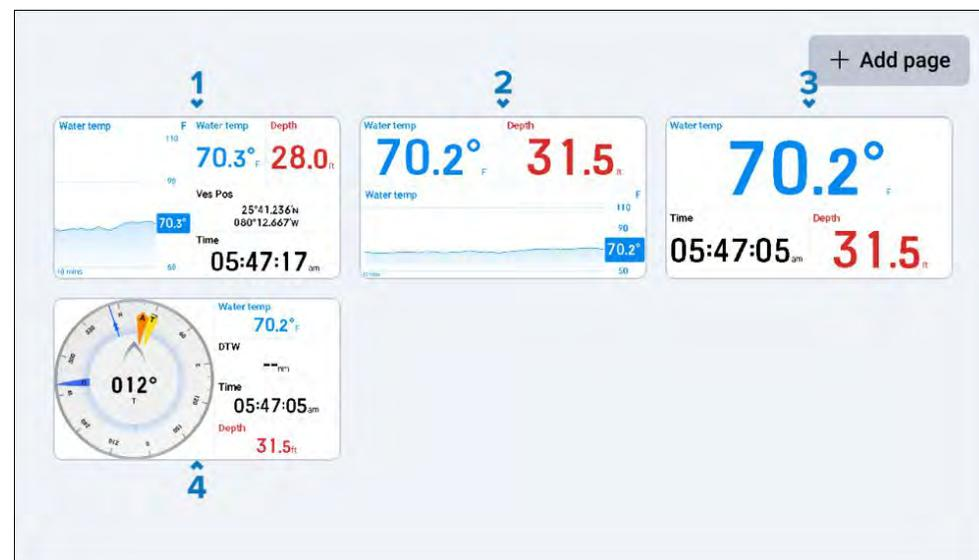
1. *[Multi-data]* — Includes 4 fishing orientated widgets and an enlarged *[Water temp]* graph widget.
