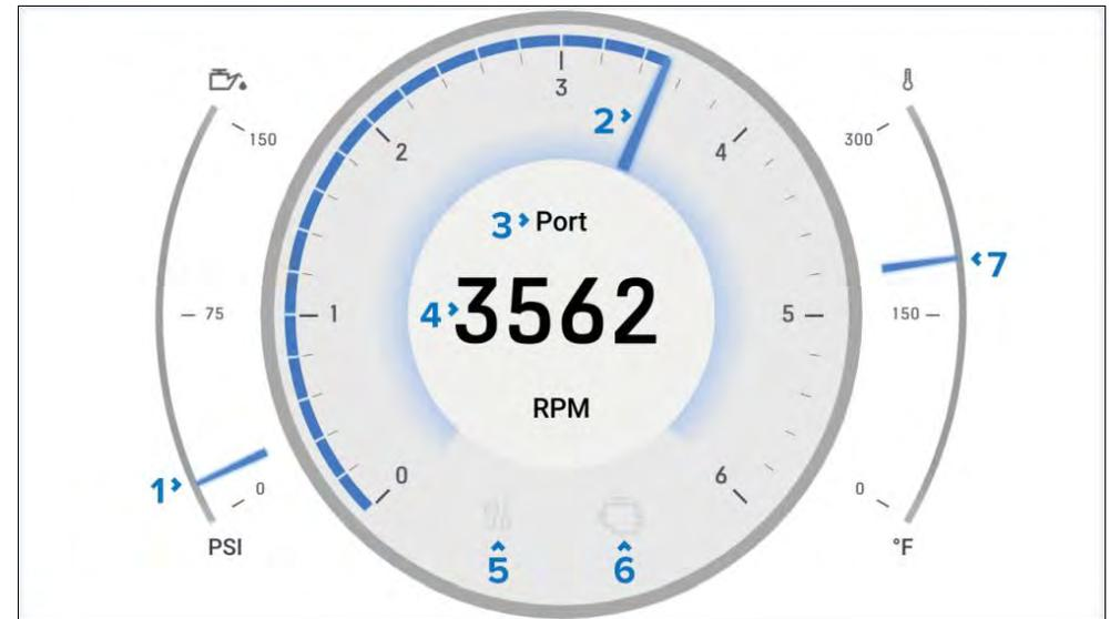
1. **Oil pressure indicator** — Current engine oil pressure indication.
