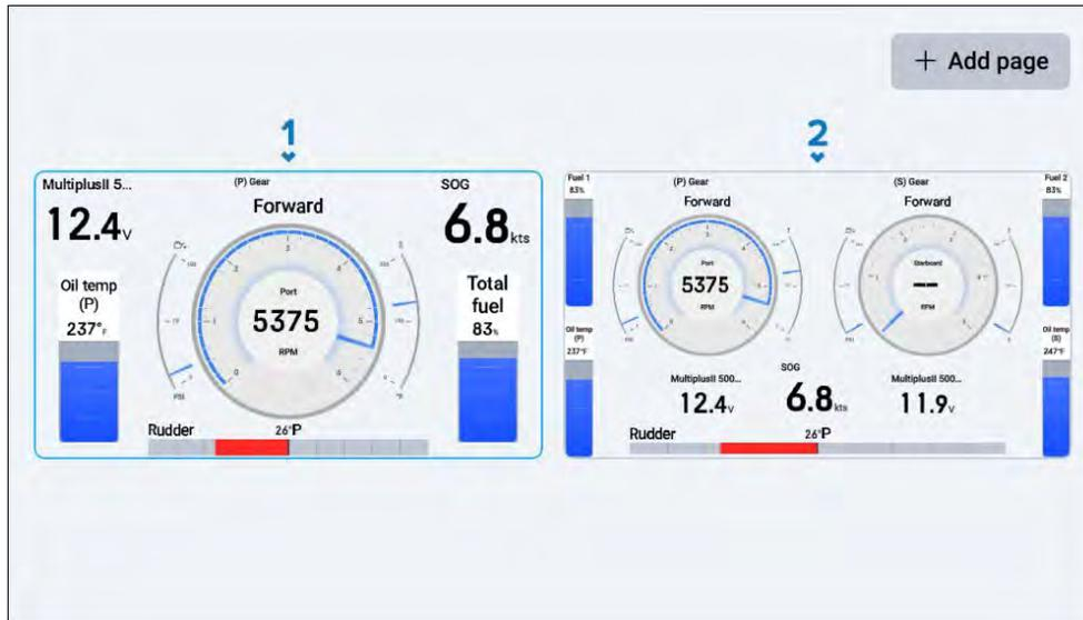
1. *[Single engine]* — Includes 6 engine orientated widgets and a center enlarged *[Engine combo gauge]* widget.
